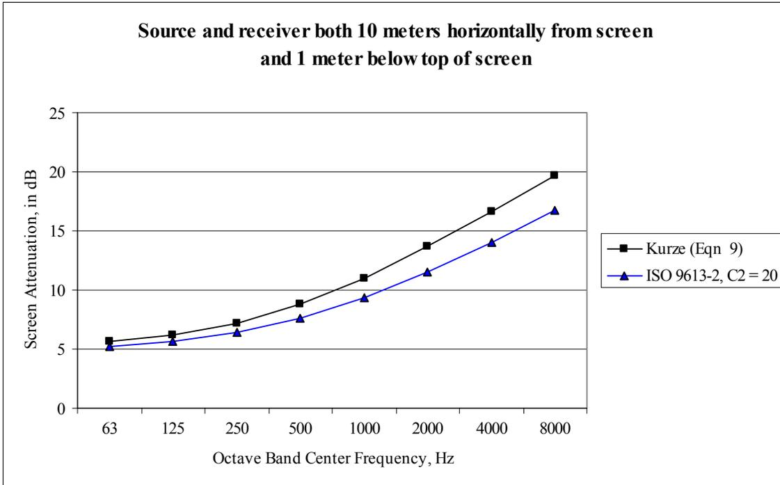
**Figure 3. Effect of ISO 9613-2 Screening Ground Term  $C_2$**
