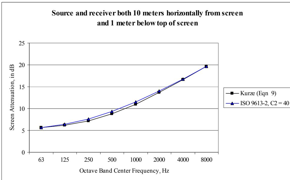
Figure 2. Comparison of ISO 9613-2 Screening Formulation and Kurze Formulation that Neglects Ground and Meteorological Effects
